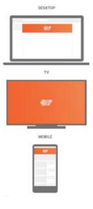
The **safe area**, where the text and logos are guaranteed to be shown is within the centre rectangle, as shown on the diagram below (1546 x 423px), this is the area that you should keep your most critical information and images to ensure they are not cut off on smaller devices.
